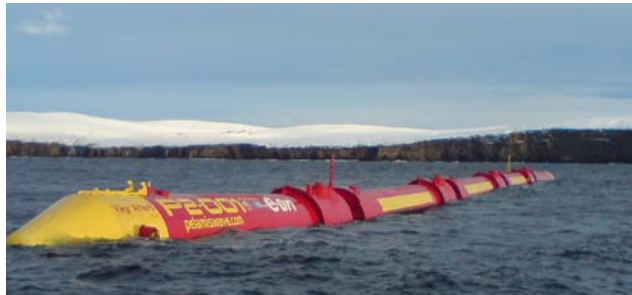
Pelamis P2 testing at EMEC
